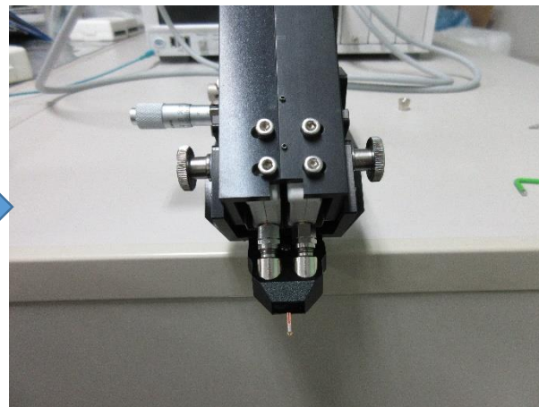
5. Connect N1055A to probe
